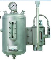
Thermosyphon Systems provide lubricant, dissipate heat and maintain the required pressure gradient across the seal faces in case of double back to back and tandem seal arrangements for pumps and agitators
